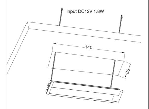
Cut hole 36 mmH x 140mmL. Connect cable either directly to 12V DC Superlux SLED driver or connect to SLED-PREWIRE cable.
