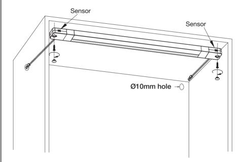
Ensure that the light fixture is installed within the 10cm detection range and is at least 5mm away from the cupboard door. Then Fix in place either directly using the two counter sunk holes in the fixture or by using the mounting brackets supplied. If required a 10mm hole can be made to feed the cables and plugs through to connect to the driver.
