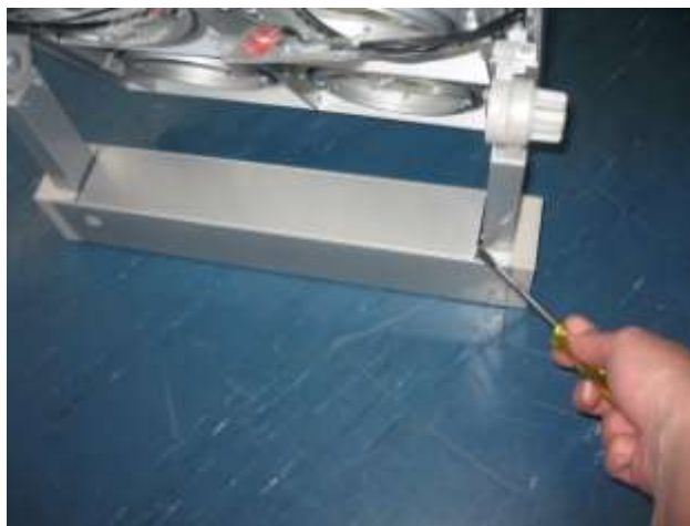
To get to wiring enclosure gently lever of panel with a flat head screw driver
